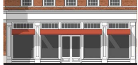
Figure 18.7 Example of signage incorporated into a storefront.
