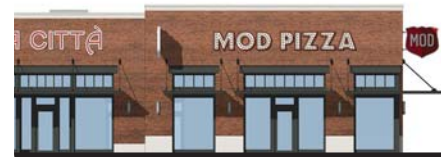
Figure 18.11 An example of a storefront with articulated bays and approximately minimum transparency.
