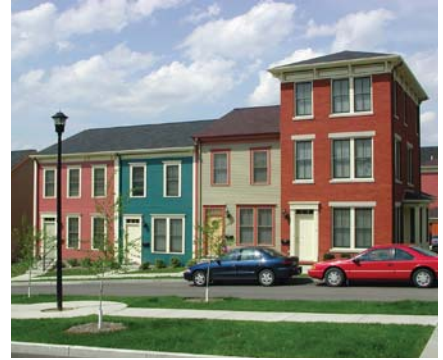
Figure 15.22 Examples of townhouses that utilize vertical articulation to visually break down the scale of the building.
