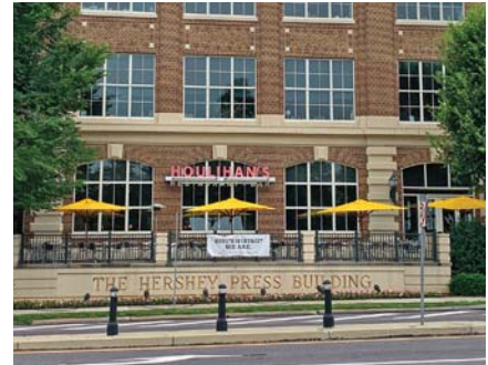
Figure 20.3 Low walls around a raised terrace retain visibility while distinguishing private from public spaces.
